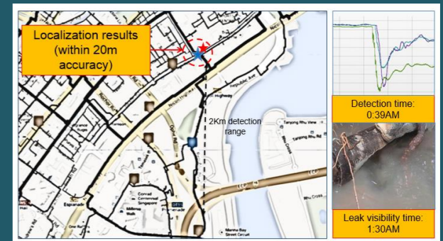
300mm (12") Ductile Iron pipe burst detected and localized
